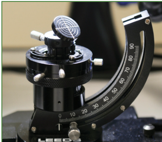
The articulating wax platen is used for mounting a small sample to Leeds Universal Holder, allowing great range of motion through a ball and socket joint design.
